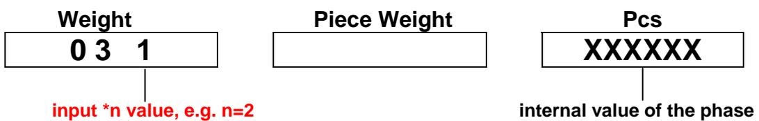
⑤ Add the 3<sup>rd</sup> weight mass (e.g. 12kg, in sum 21kg) and input \*n value (e.g. \*n=4), then press  key
