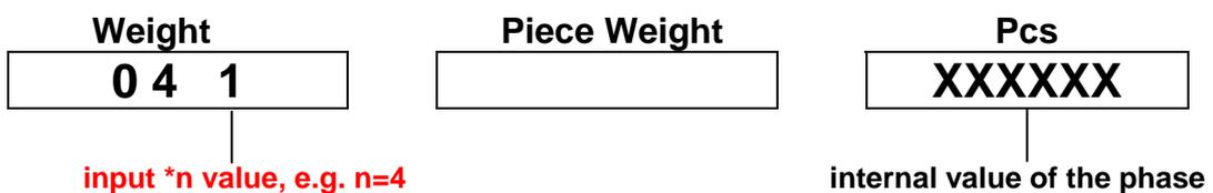
⑥ Add the 4<sup>th</sup> weight mass (e.g. 12kg, in sum 33kg) and input \*n value (e.g. \*n=4), then press  key
