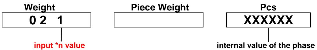
④ Add the 2<sup>nd</sup> weight mass (e.g. 6kg, in sum 9kg) and input \*n value (e.g. \*n=2), then press  key
