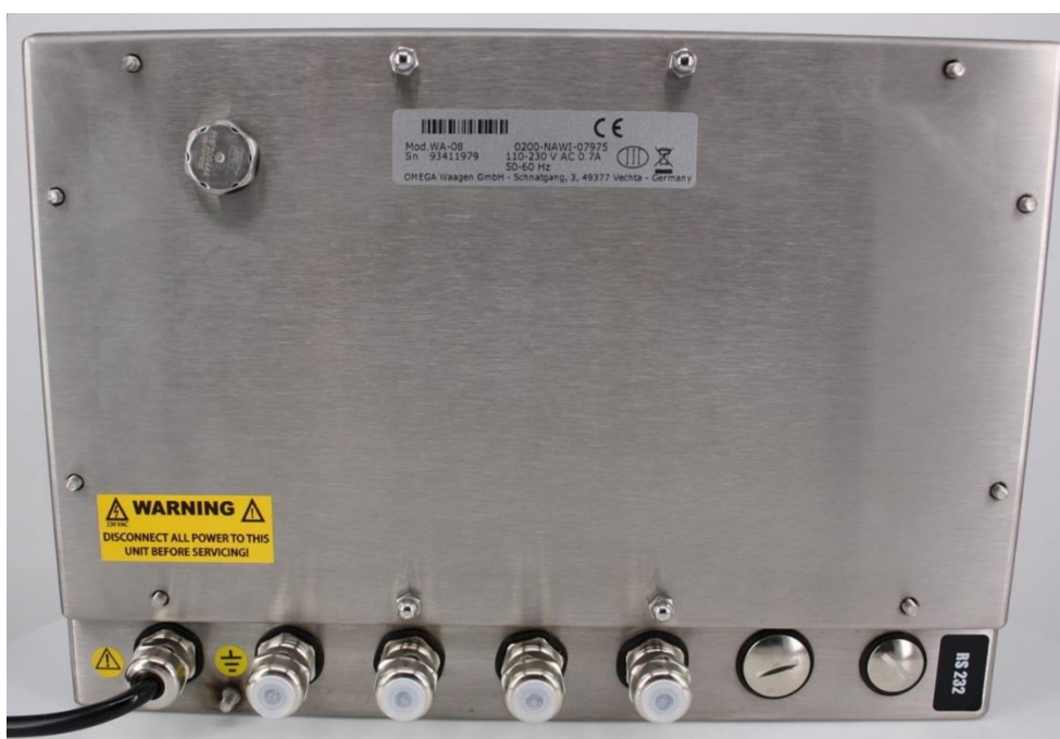
Figure 3 WA-08 indicator rear view.
